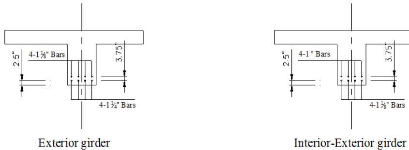
Figure 16 Reinforcement arrangement in girders
