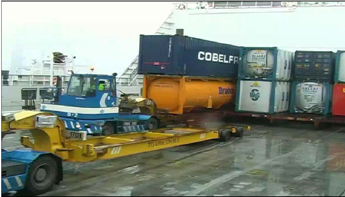
Figure 11 The cassette system (Source: TTS, 2013)
