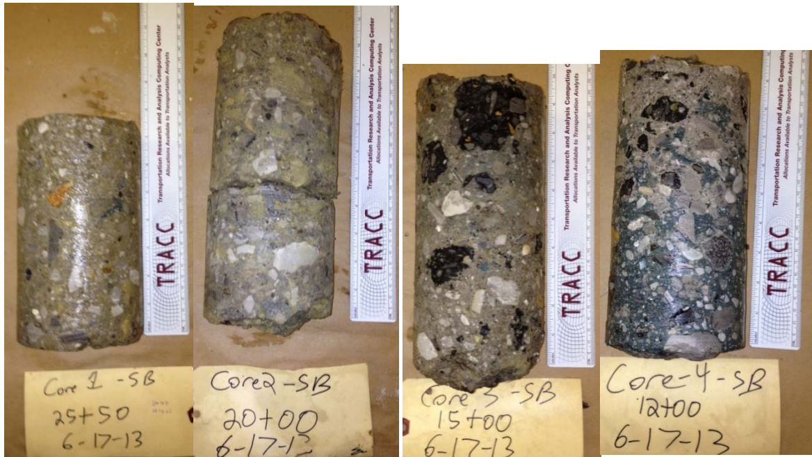
Figure 20 Southbound cored samples
