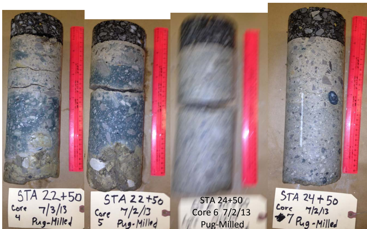
Figure 26 NB-Pug cored samples – Round 2
