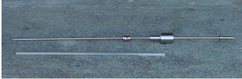
Figure 2 Dynamic cone penetrometer (DCP)
