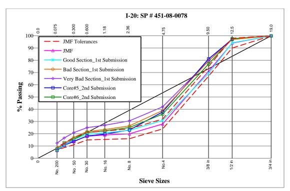
Figure 41 Aggregate blended gradations
