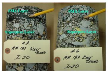
Figure 40 Aggregate arrangement in the SMA mixture
