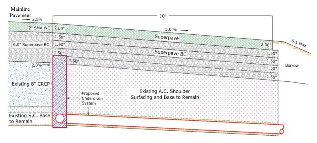
Figure 26 New proposed cross sections showing edge drain
