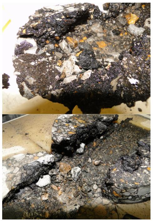
Figure 32 Moisture damage observed on cores after LWT test
