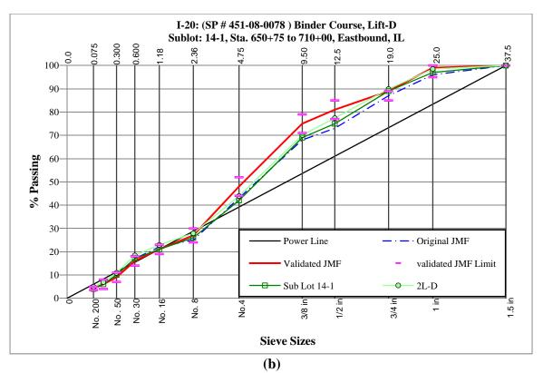
Figure 29 Comparisons of blended aggregate gradations for sublots 4-1 and 14-1
