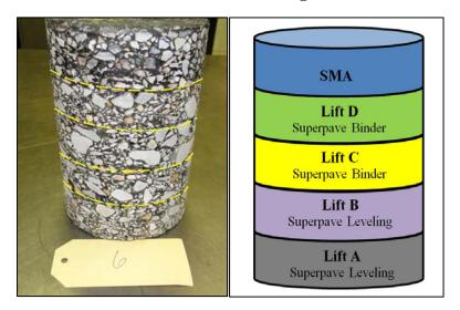
Figure 5 Layers in a roadway core
