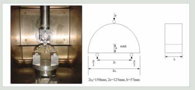
Semi circular bend test setup and specimen configuration
