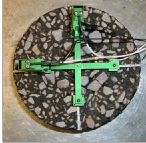
Figure 4 DCSE test sample instrumentation
