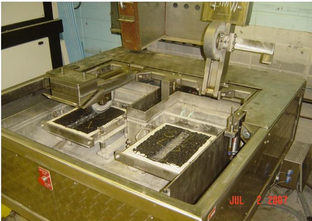
Figure 9 Hamburg loaded wheel tracking device
