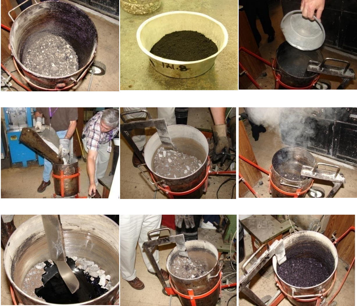
Figure 2 HMA mix blending procedure
