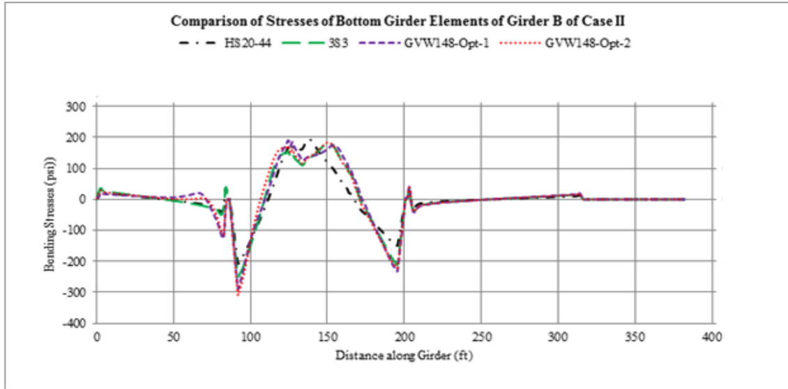
Figure 59 Comparison of bending stress distribution of bottom elements - Girder B of Case II
