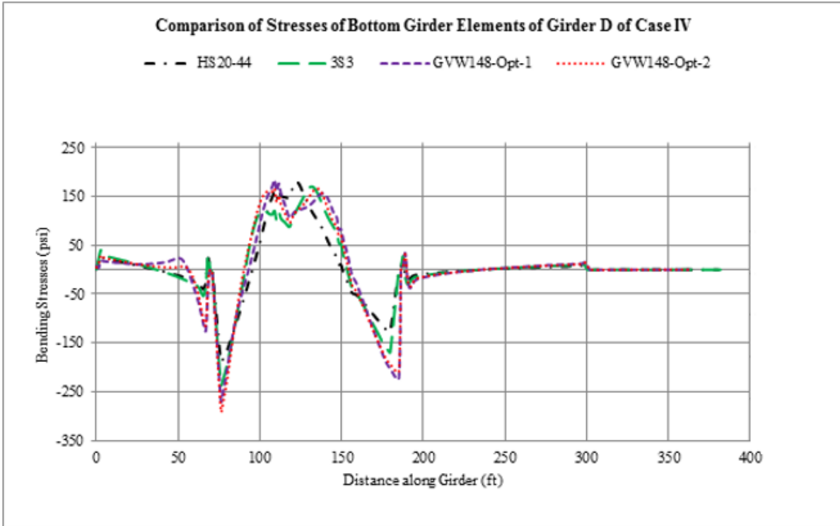
Figure 83 Comparison of bending stress distribution of bottom elements - Girder D of Case IV
