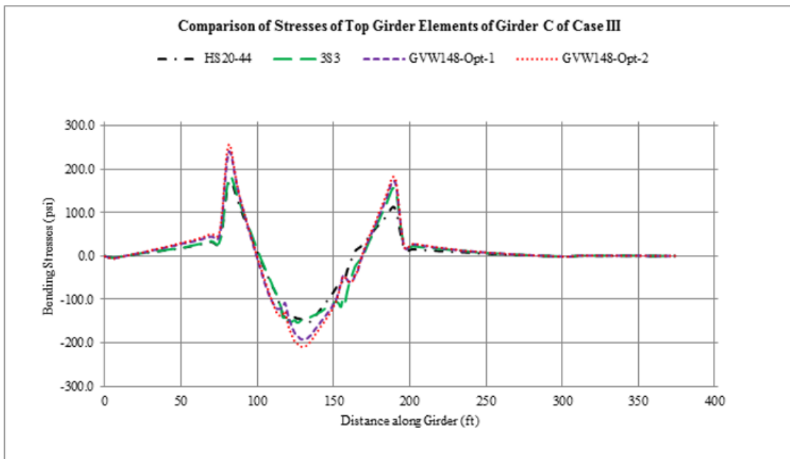
Figure 74 Comparison of bending stress distribution of top elements - Girder C of Case III
