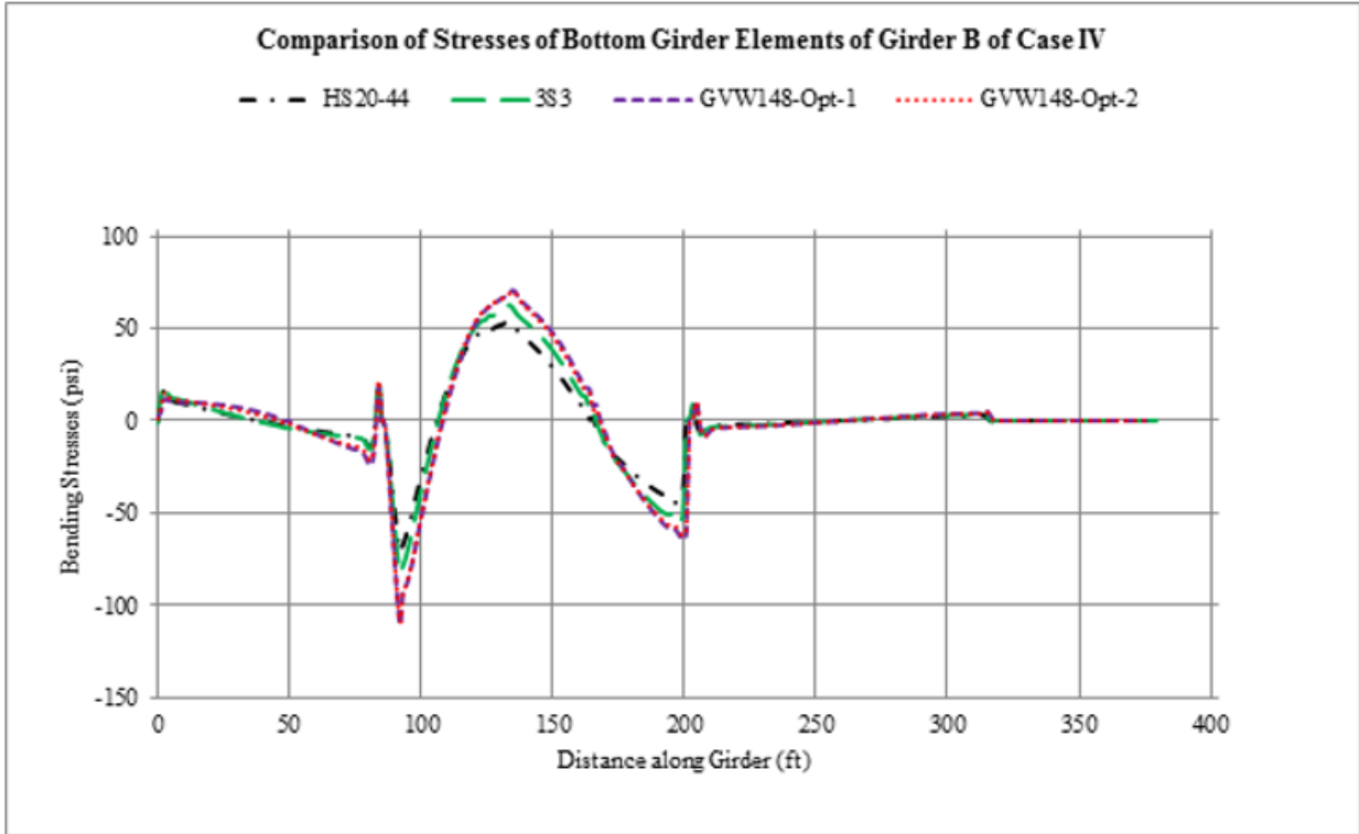
Figure 79 Comparison of bending stress distribution of bottom elements - Girder B of Case IV
