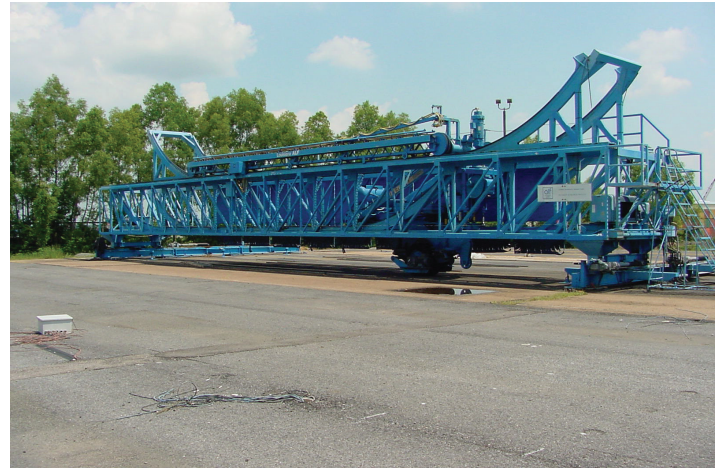
LTRC’s Accelerated Loading Facility
