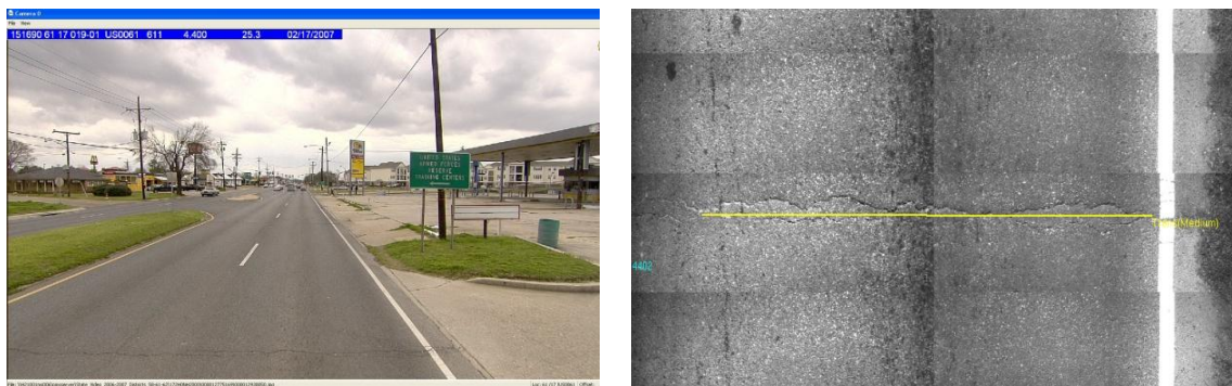
Figure 12 Pavement imaging and the detection of reflective cracking
