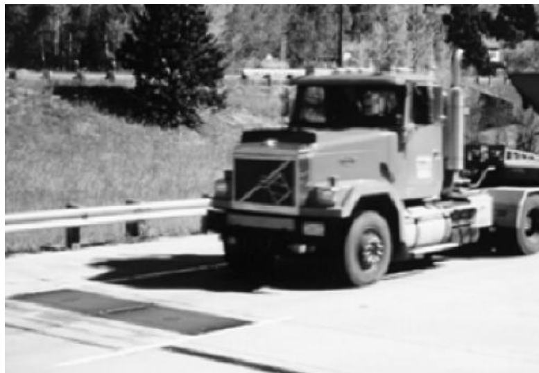
Figure 8 Single load cell (source: International Road Dynamics Inc., www.irdinc.com )
