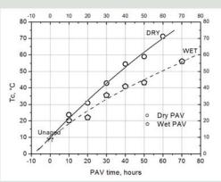
Figure 2 Variation of critical temperature of multiple PAV dry-aged and wet-aged PMAC samples
