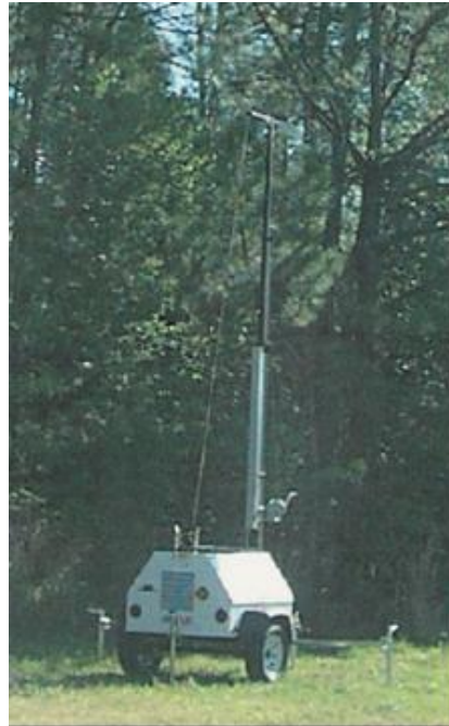
Figure 12 RTMS device mounted on trailer (Santa Fe Technologies)
