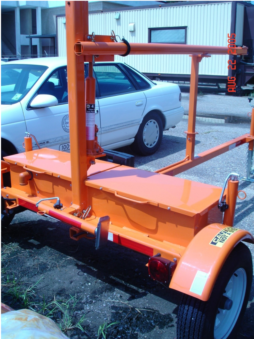
Figure 25 RTMS trailer (right-side view)
