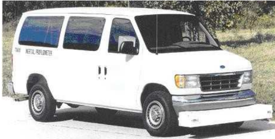
a. Mini-van with laser and inertial sensors
