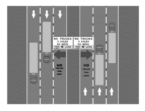
Figure 1 Left lane truck restriction on a three lane highway (Harwood et al., 2003)
