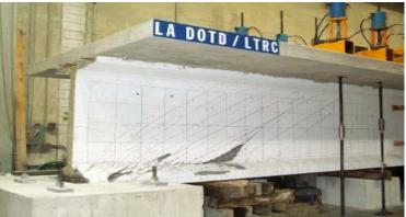
Shear Test at CTL
