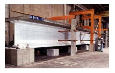
Fatigue Test Setup
