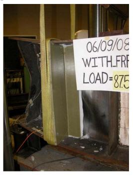
(b) Stiffened specimen Figure 17 Failure of beam specimens
