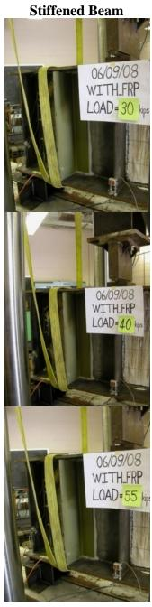
Figure 16 Progression of loading for beam specimens
