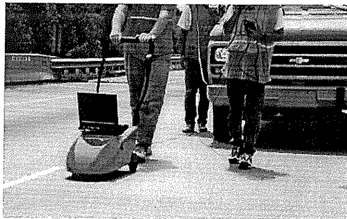
Figure 11b A walking profiler test on I-310
