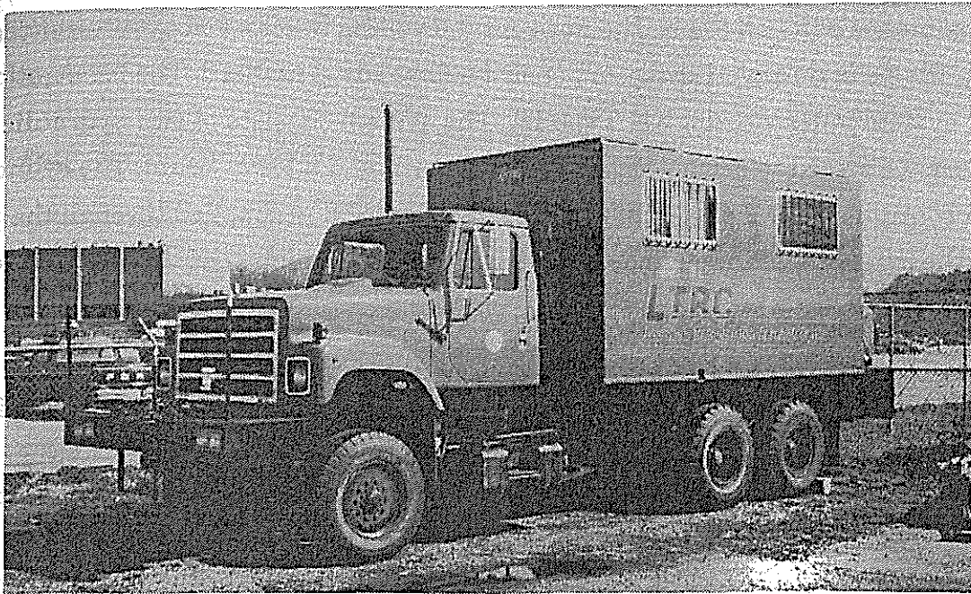
Figure 1a. General Exterior View of Louisiana Electric Cone Penetrometer System (LECOPS)
