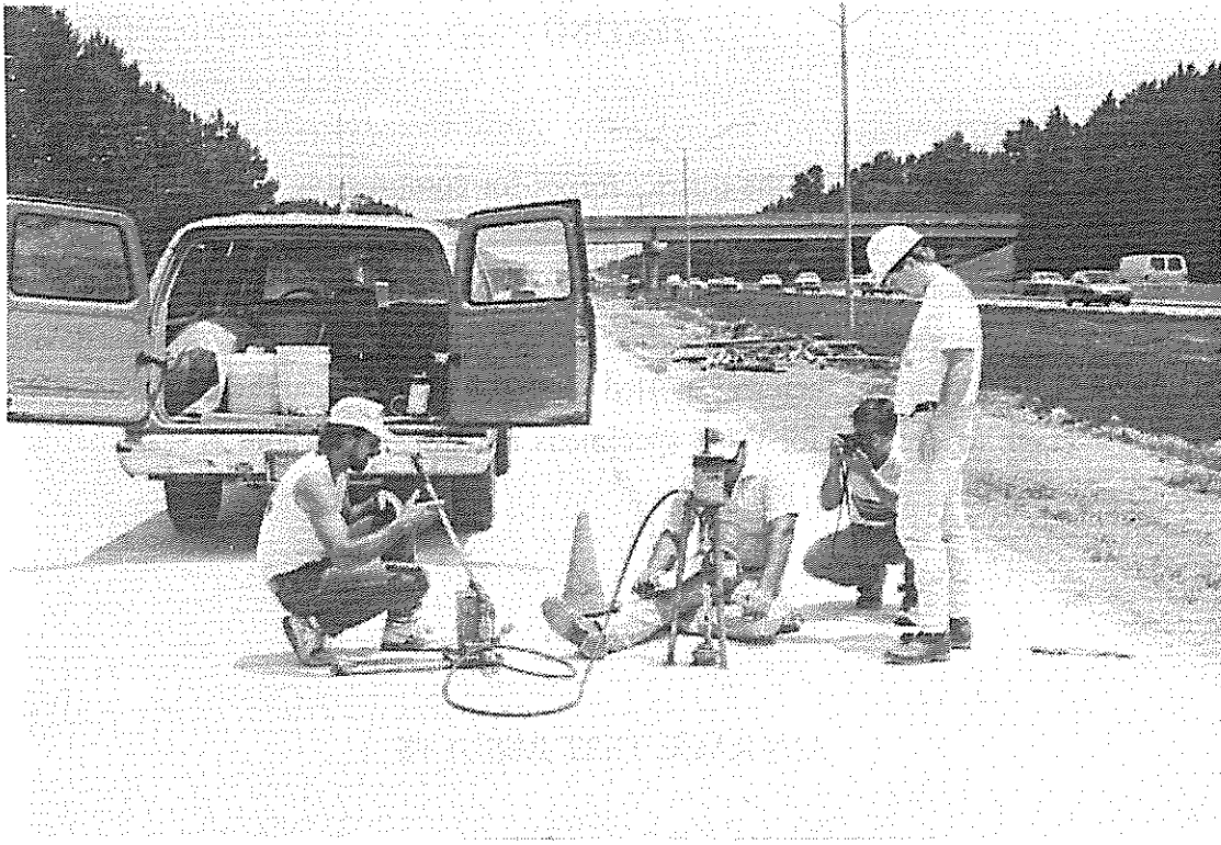
Figure 5. ACI pull test in the field.
