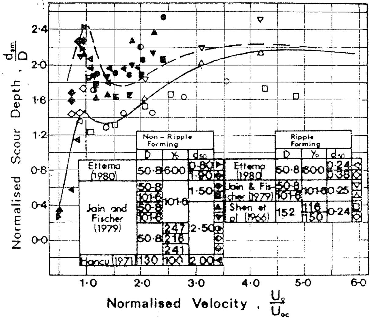
Figure 4. Maximum Scour Depth as a Function of Mean Flow Velocity For Relatively Deep Flows, Comparison With Data by Other Investigators (10)
