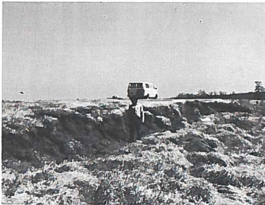
Figure 11. Failures are slump-earthflows which are separated by an earthflow. This slope is located in the I-20 study area, Tendal northeast quadrant, Locality N15, Madison Parish.
