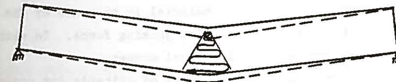
(c) Near the completion of heating the movement is reversed and the damage is increased
