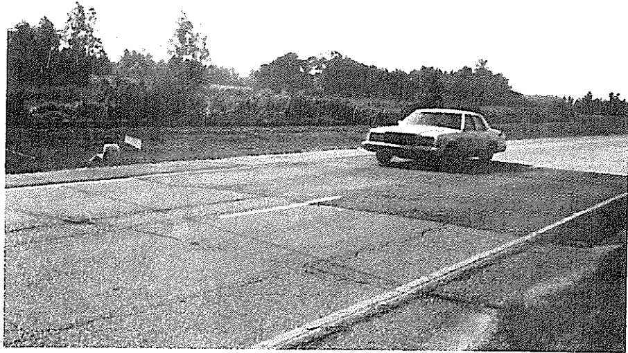
Rough Concrete Test Section on La. 23 in South Louisiana. 4200-Pound Sedan Making Test Run.
