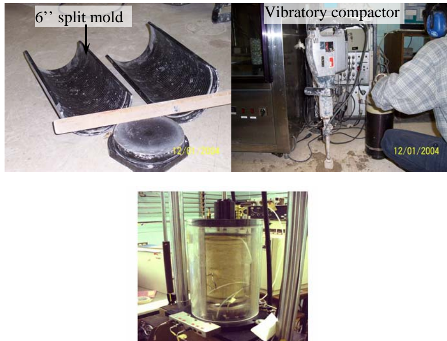
Figure 6 Compaction of stabilized BCS with entire gradation
