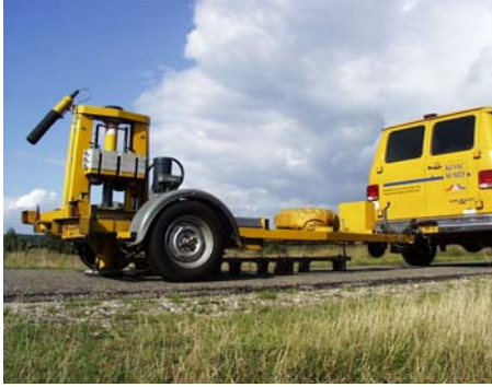
Figure 13 Dynatest 8002 falling weight deflectometer
