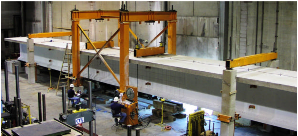
Figure 17 Flexural strength test setup
