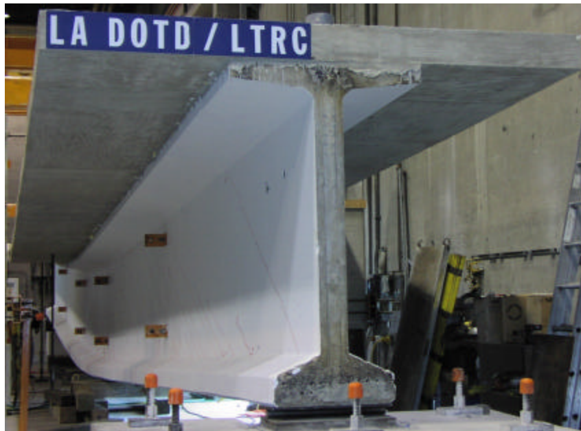
Figure 21 Specimen BT12 prior to completion of the flexural strength test
