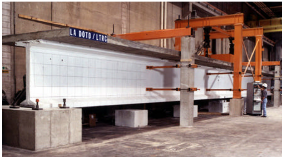
Figure 6 Fatigue test setup
