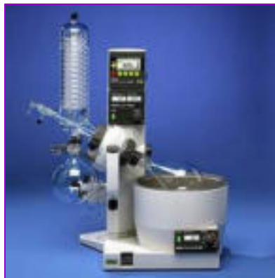
Figure 4 Rotary evaporator for concentration of toluene asphalt extracts
