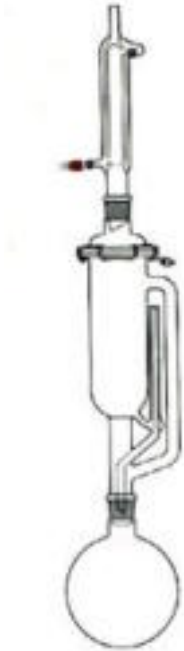
Figure 3 Soxhlet apparatus for extraction of asphalt using toluene
