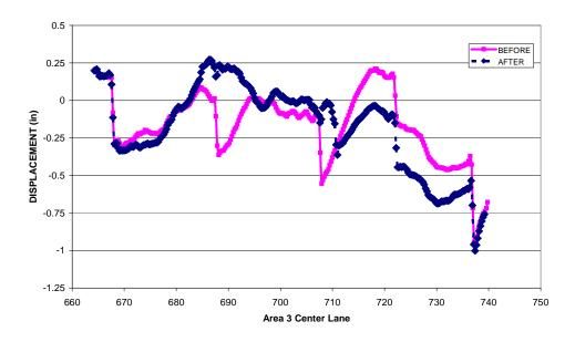
Figure 91 Profile from high speed profiler area 3 center lane
