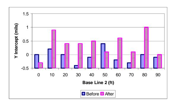
Figure 108 FWD potential void detection for base line 2
