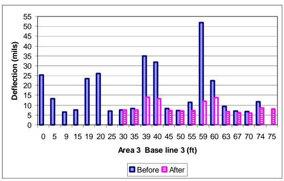
Figure 57 FWD first sensor deflections (16 kips) area 3 base line 3
