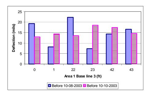
Figure 20 FWD first sensor deflections (comparison before and after rainfall)
