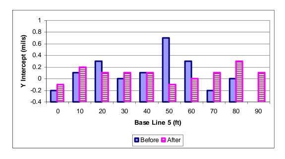
Figure 110 FWD potential void detection for base line 5
