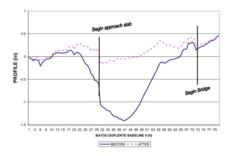
Figure 32 Walking Profiler Bayou Duplente SB base line 5
