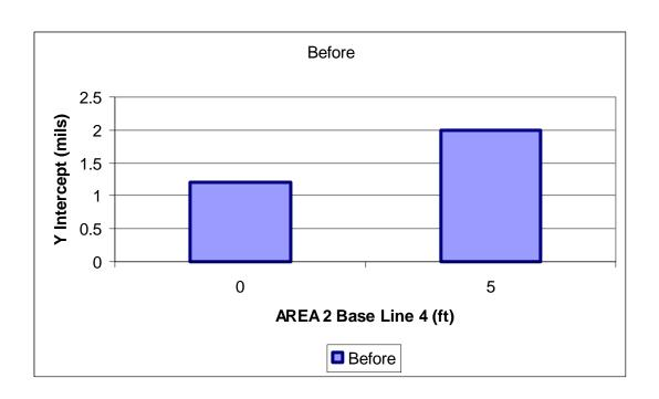
Figure 66 FWD potential void detection for area 2 base line 4
