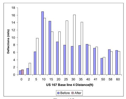
Figure 125 FWD first sensor deflections US 167 base line 4
