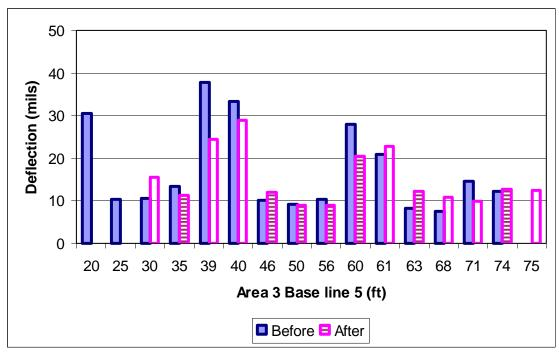
Figure 59 FWD first sensor deflections (16 kips) area 3 base line 5
