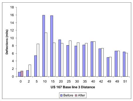
Figure 124 FWD first sensor deflections US 167 base line 3
