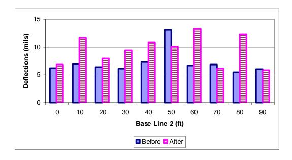
Figure 104 FWD first sensor deflections for base line 2
