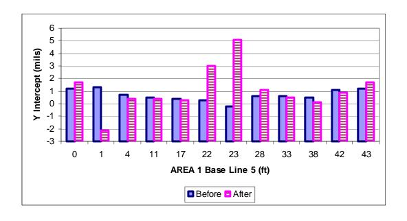
Figure 63 FWD potential void detection for area 1 base line 5
