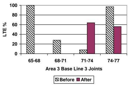
Figure 24 Load transfer efficiency for Area 3 Base Line 3
