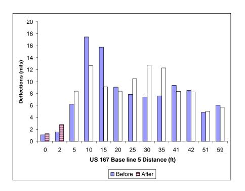
Figure 126 FWD first sensor deflections US 167 base line 5
