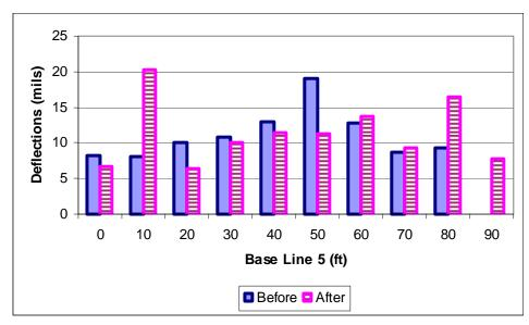
Figure 106 FWD first sensor deflections for base line 5
