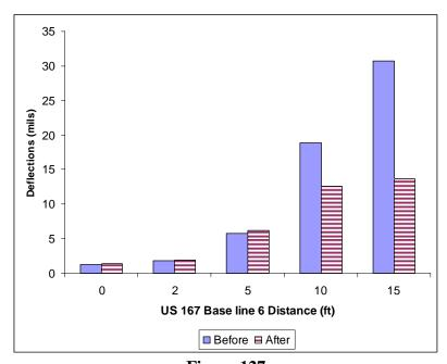
Figure 127 FWD first sensor deflections US 167 base line 6
