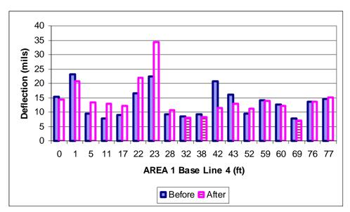
Figure 50 FWD first sensor deflections (16 kips) area 1 base line 4
