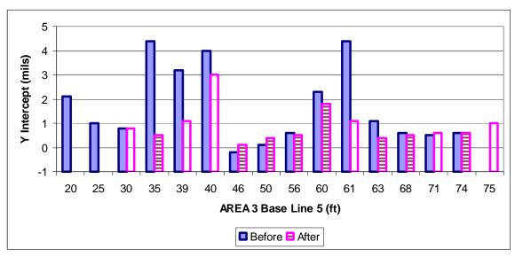
Figure 71 FWD potential void detection for area 3 base line 5
