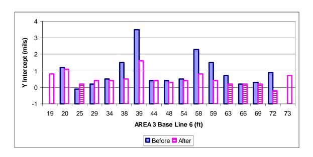
Figure 72 FWD potential void detection for area 3 base line 6
