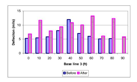
Figure 105 FWD first sensor deflections for base line 3
