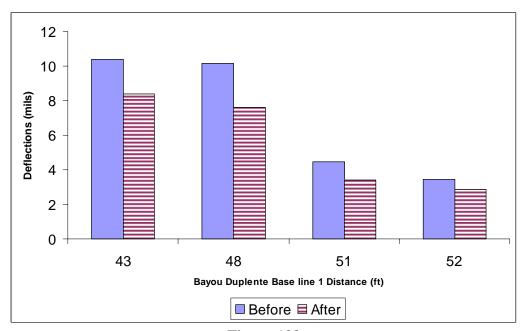
Figure 133 FWD first sensor deflections Bayou Duplente base line 1
