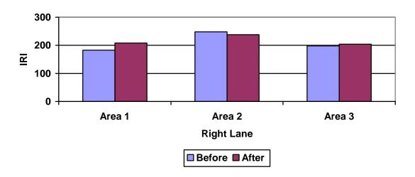
Figure 97 IRI from high speed profiler areas 1, 2, and 3 right lane
