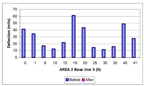
Figure 55 FWD first sensor deflections (16 kips) area 2 base line 5
