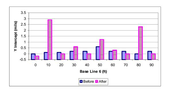
Figure 111 FWD potential void detection for base line 6
