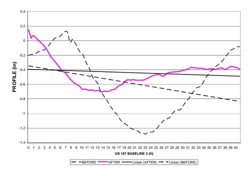
Figure 121 High speed profiler US 167 NB baseline 3
