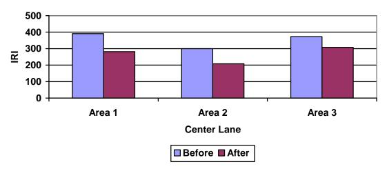
Figure 95 IRI from high speed profiler areas 1, 2, and 3 center lane
