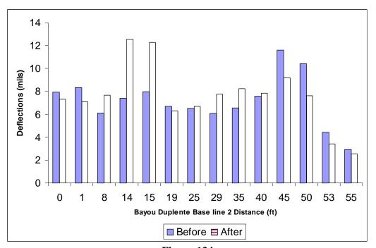
Figure 134 FWD first sensor deflections Bayou Duplente base line 2
