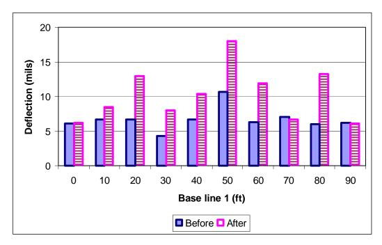
Figure 10 FWD first sensor deflections (14,500 lb load)
