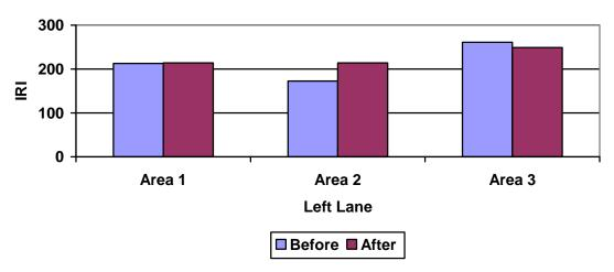
Figure 93 IRI from high speed profiler areas 1, 2, and 3 left lane
