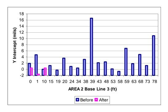
Figure 65 FWD potential void detection for area 2 base line 3
