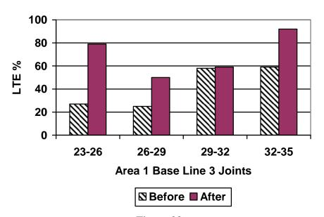
Figure 23 Load transfer efficiency for Area 1 Base Line 3
