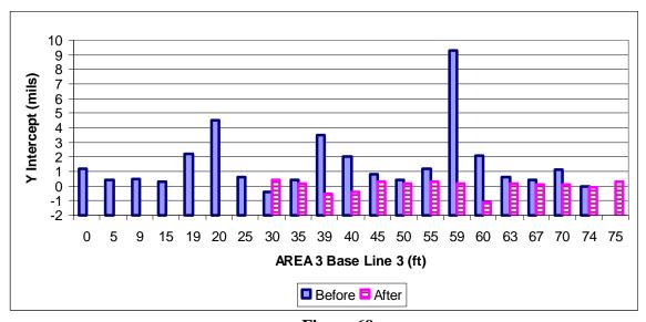
Figure 69 FWD potential void detection for area 3 base line 3
