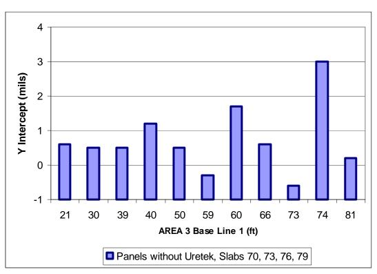
Figure 73 FWD potential void detection for area 3 base line 1
