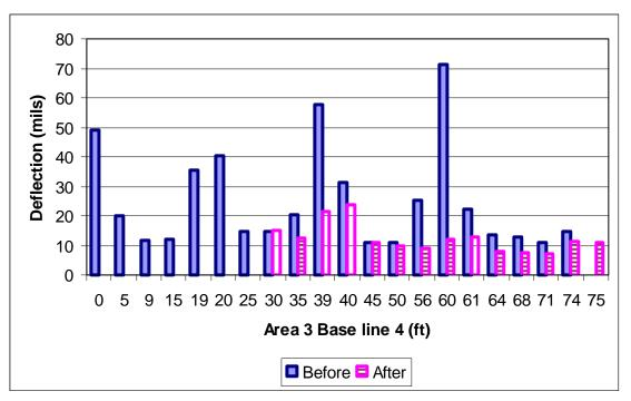
Figure 58 FWD first sensor deflections (16 kips) area 3 base line 4
