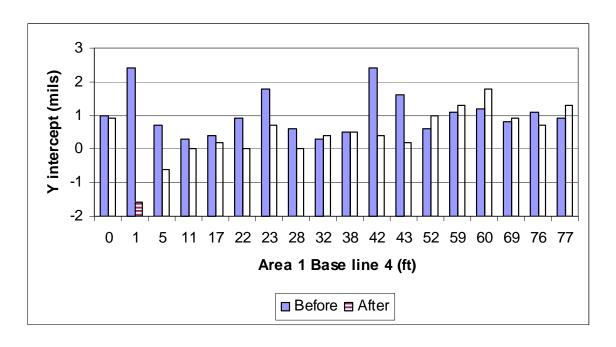
Figure 62 FWD potential void detection for area 1 base line 4
