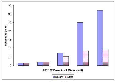
Figure 123 FWD first sensor deflections US 167 base line 1
