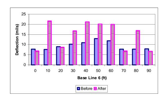
Figure 107 FWD first sensor deflections for base line 6
