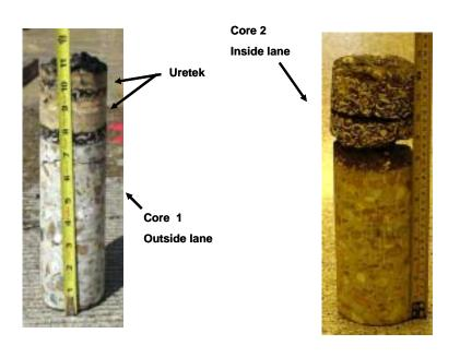
Figure 14 Concrete cores
