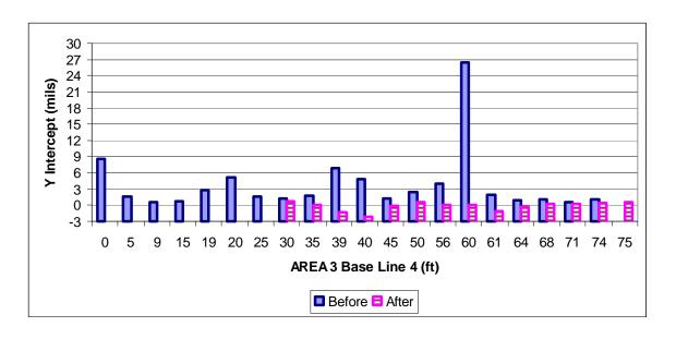
Figure 70 FWD potential void detection for area 3 base line 4
