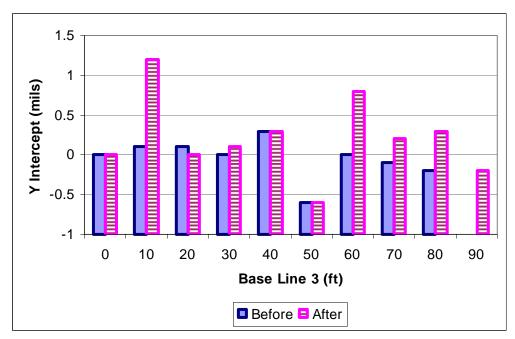
Figure 109 FWD potential void detection for base line 3
