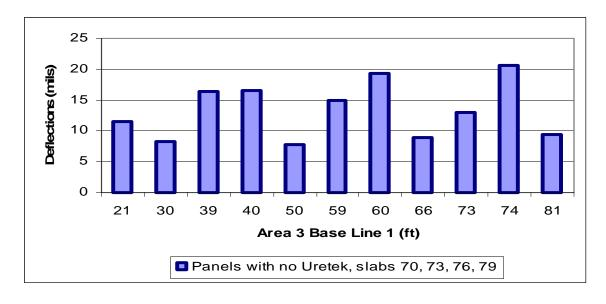
Figure 61 FWD first sensor deflections (16 kips) area 3 base line 1
