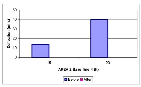
Figure 54 FWD first sensor deflections (16 kips) area 2 base line 4
